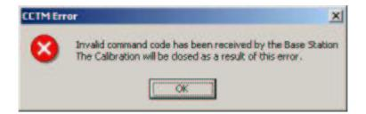
Selecting okay causes to Calibration Kit to disconnect from the TB8100 Base Station
